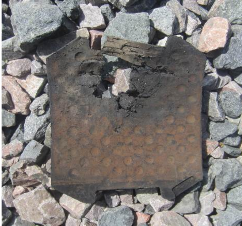
Figure 2.2 Example of tearing as a failure mode of rail pad assemblies
