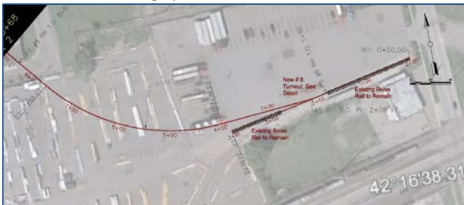
Figure 3 - Horizontal curve to new warehouse site
