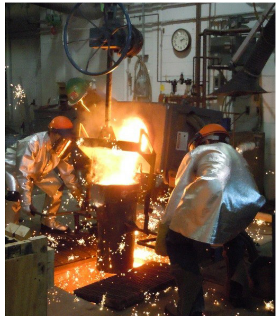
Magnesium nodularizing treatment of 300 lbs of ductile iron in the Michigan Tech Foundry. Magnesium treatment is the critical step to make the round graphite nodules characteristic of ductile iron.
