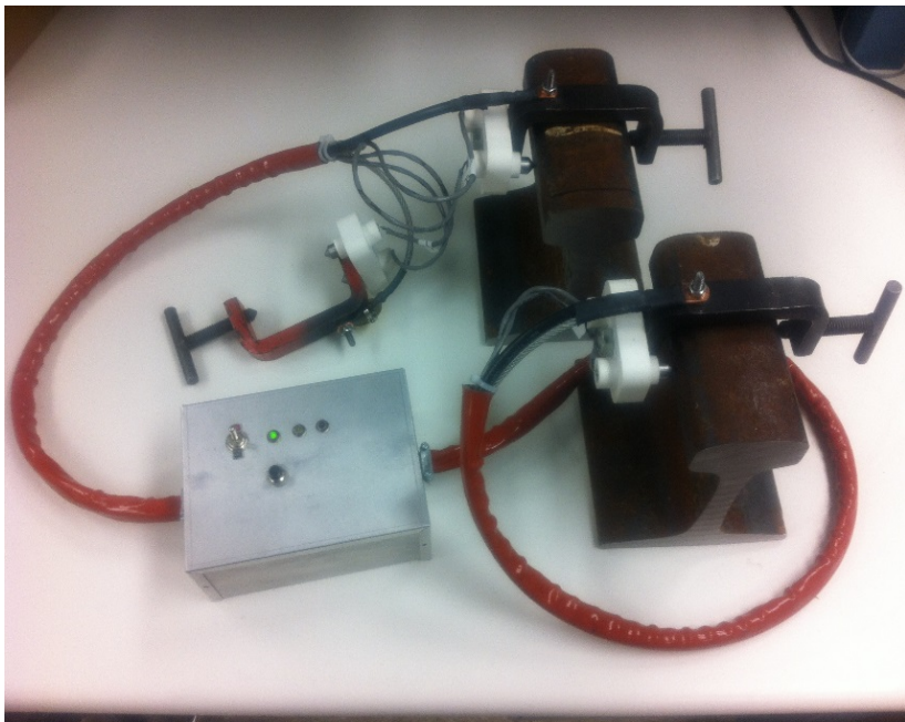
Figures 2 and 4 - Rail shunt testing device (left), Student working the device (right)
