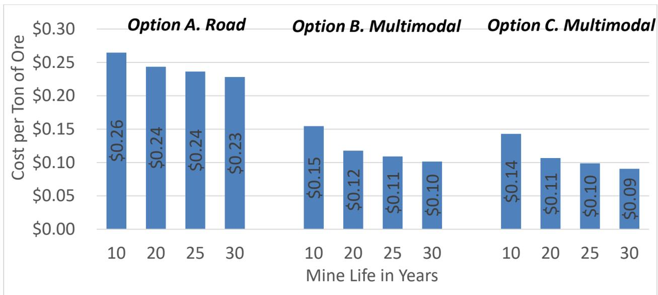
Figure 7: Emission Costs per ton of Ore Transported
