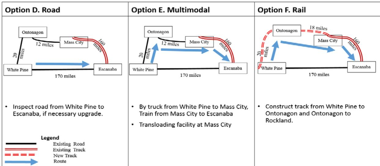
Figure 3: Infrastructure and Route Comparison of Concentrate Transportation Options between White Pine and Escanaba
