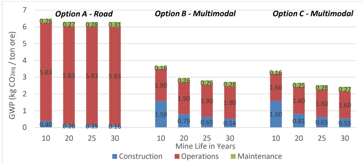
Figure 5: Kg of CO<sub>2</sub>eq per ton of Ore Transported for Different Options and Mine Life Times
