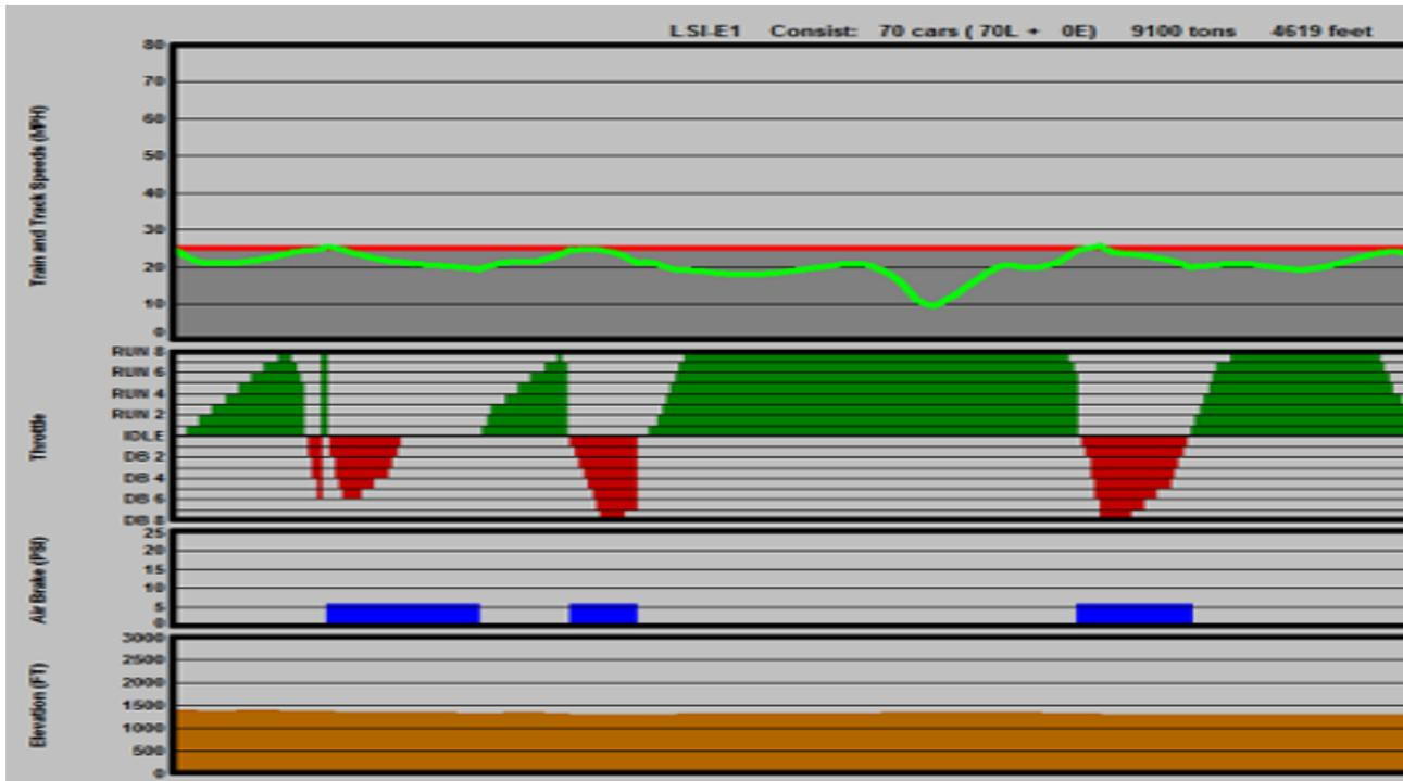
Figure 4: Screen shot of RTC Simulation including the Train Speed, Throttle, Braking and the Track Elevation from Top to Bottom
