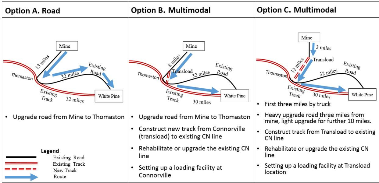
Figure 2: Infrastructure and Route Comparison of Ore Transportation options between the Mine and White Pine
