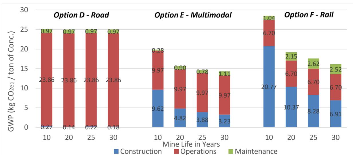
Figure 6: Kg of CO<sub>2</sub>eq per ton of Concentrate Transported for Different Options and Mine Life Times
