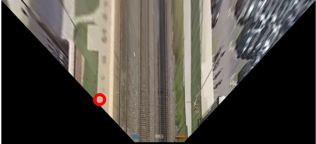
Fig. 4: Video frame after perspective transformation
